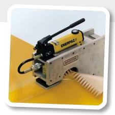
The 1st punching process can begin, i.e. close the rotary valve and bring the unit to pressure by operating the hydraulic pump.
